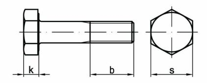
High-Strength Structural Bolts (HV) in stainless steel and carbon and alloy steel.
